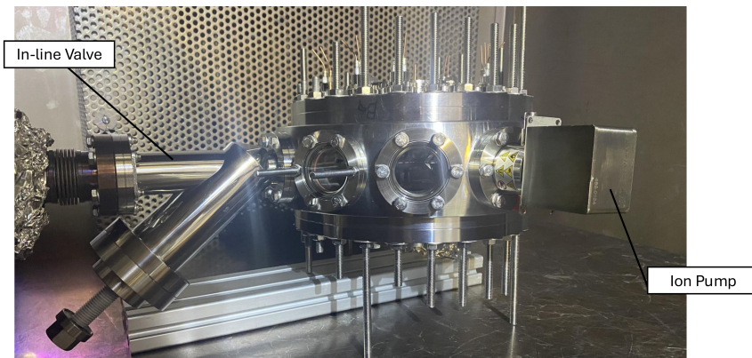
Figure 4.6.: Closed trap chamber inside the oven. The in-line valve is connected to a pumping station located to the left (not pictured), which pumps down the system as the trap is being baked. The trap was baked at 250\text{ }^{\circ}\text{C} for one week until reaching a pressure lower than 2 \times 10^{-11}\text{ mbar} .
