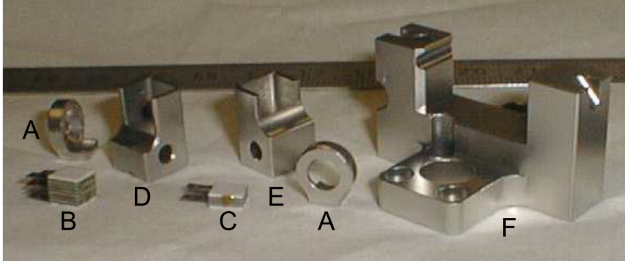
Figure 4.7: Components of the cavity mount: mirror frames (A), slow PZT stack (B), fast PZT stack (C), pillar for the slow PZT stack (D), pillar for the fast PZT stack (E) and frame (F).
