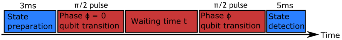
Figure 3.15: Experimental sequence of the Ramsey measurement. The sequence starts with 3 ms of state preparation. Afterwards, the first \pi/2 pulse is applied. After a waiting time t , the second \pi/2 pulse with a phase \Phi is applied to the ion. The sequence ends with a 5 ms of state detection, following the methods described in the previous section.
