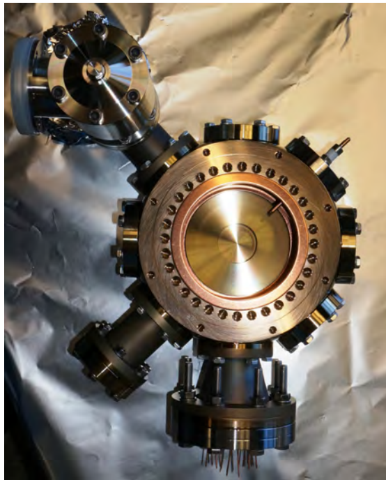
Figure 4.19: Assembled chamber prior to the vacuum bake. The orientation is the same as in the schematics in figure 4.18. The valve for connecting the chamber to an external pump is mounted on the upper left flange of the octagon, the RF feedthrough on the upper right flange and the tube for connecting the combined ion getter and NEG pump on the lower left flange, respectively. On the bottom is the conical reducer and the electrical feedthrough. For the high temperature vacuum bake the chamber was sealed with blind flanges.
