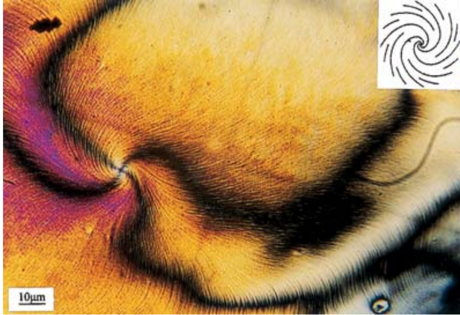
Figure 4.3: Visualization of the director field of a liquid crystal. There are various processes that allow the imaging of the director field of liquid crystals. The big black lines are results from polarizing optical microscopy and show the spatial variation of the polarization of the light propagating through the sample. In the technique applied for this image the fine lines are perpendicular to the director field and therefore allow its reconstruction. The inset in the upper right corner shows the director lines at the singularity or disclination. From [13]
