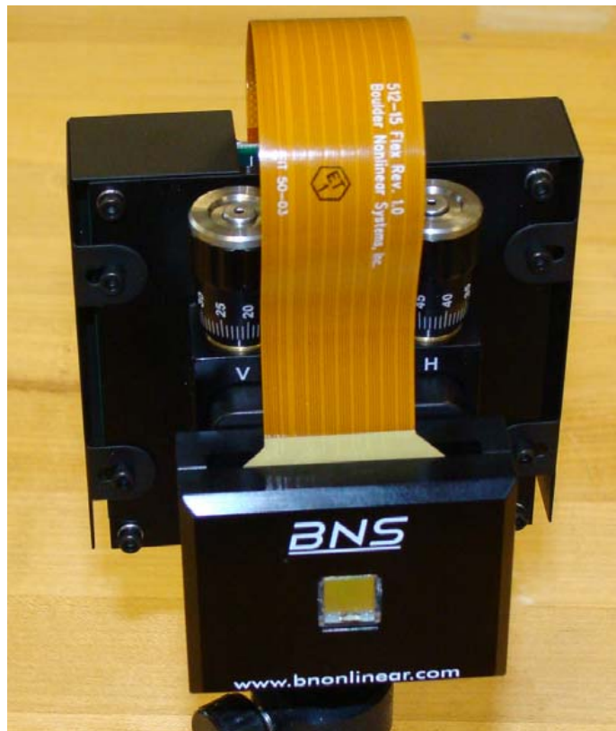
Figure 4.5: The 512 \times 512 XY-series SLM by Boulder Nonlinear Systems It features 512 by 512 pixels based on LCoS (Liquid Crystal on Semiconductor) pixels that can be addressed with 65536 levels. The small reflective area at the very front of the device is the active region, which houses the liquid crystal pixels.
